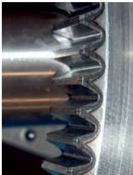
Fig. 2: Finish hardened teeth
