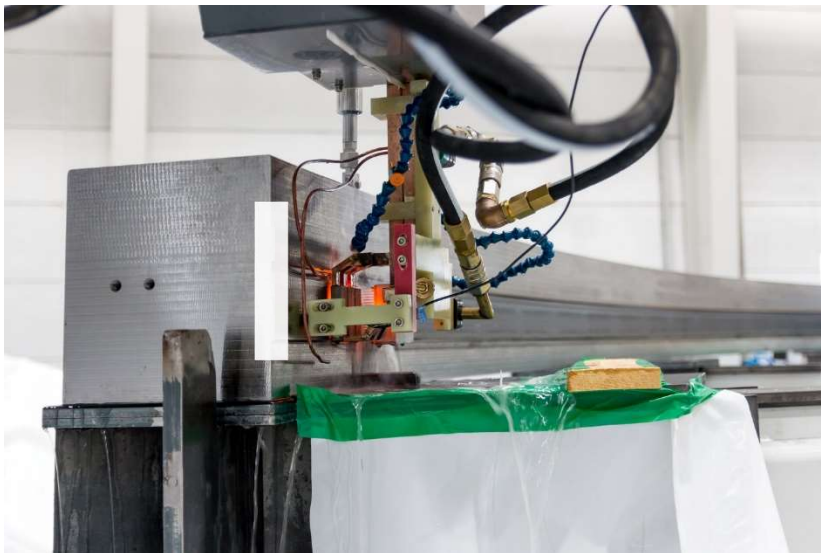
Figure 7: Hardening of a segment in the test phase
