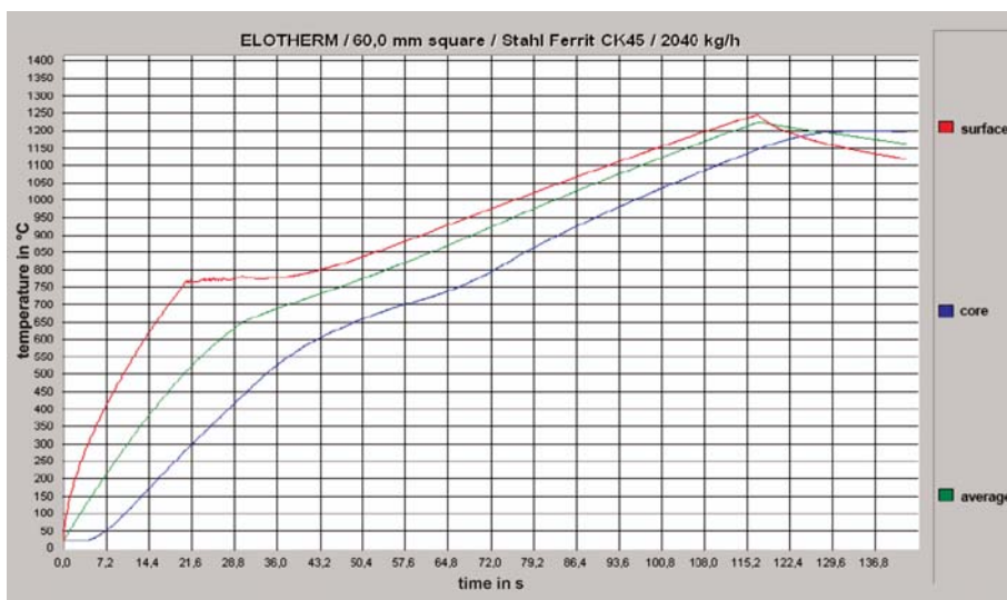
Fig. 3: Heating-up time approx. 117 s; surface temperature approx. 1250 °C
