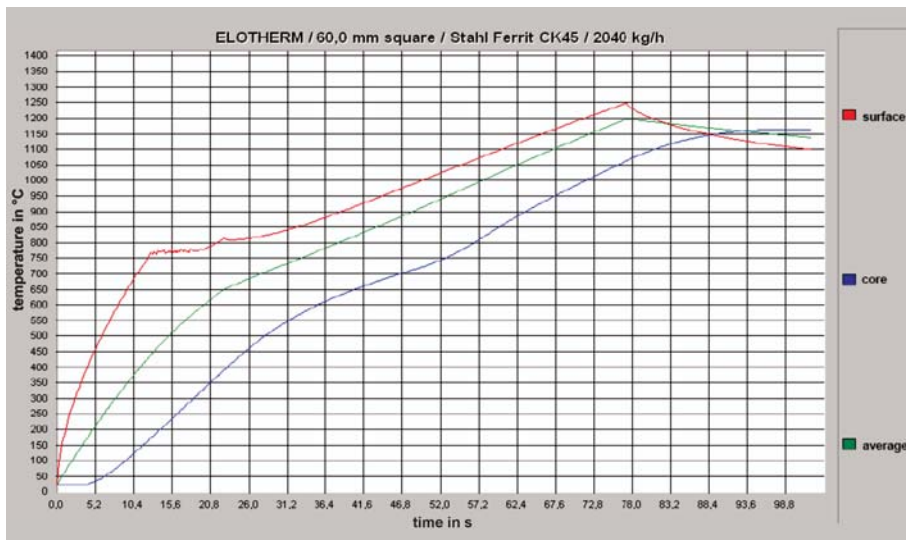
Fig. 2: Heating-up time approx. 77 s; surface temperature approx. 1250 °C
