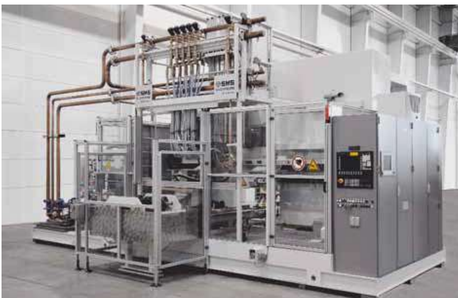
Fig. 4: Flexible hardening machine for crankshafts
