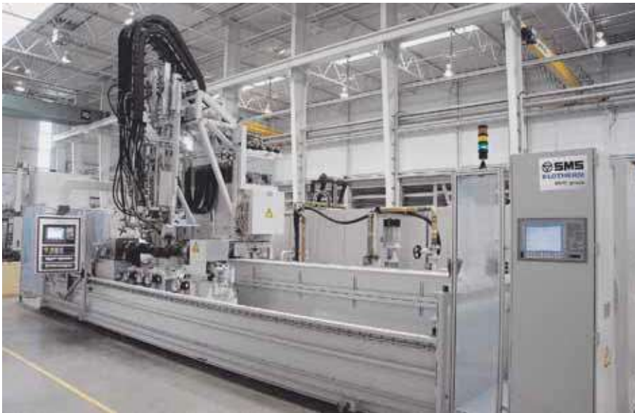
Fig. 3: Hardening machine for large crankshafts up to 5000mm in size
