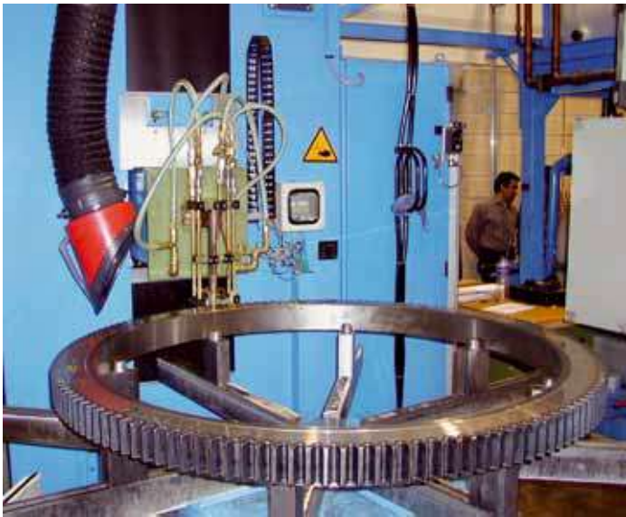
Fig. 3: Model ZHM induction hardening machine, horizontally positioned ring
