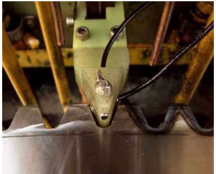
Fig. 12: Non-contact sensor for automatic inductor position control
