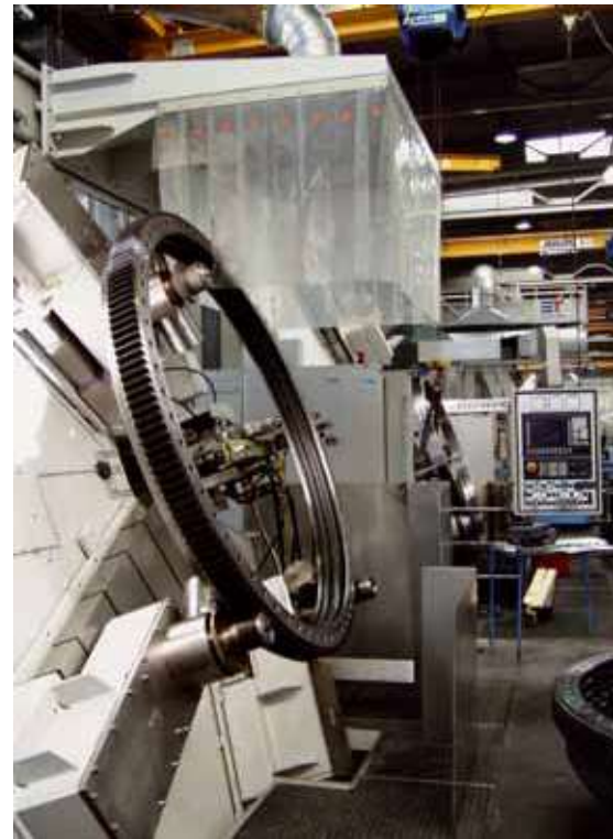
Fig. 4: Model RHM induction hardening machine, stationary tilted ring (70°)
