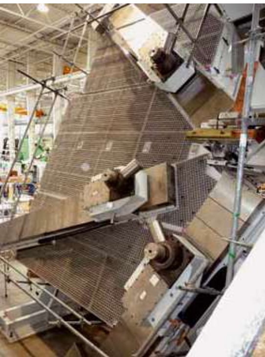
Fig. 5: Model RHM-S induction hardening machine with pre-heater & 0-70° adjustable tilt table
