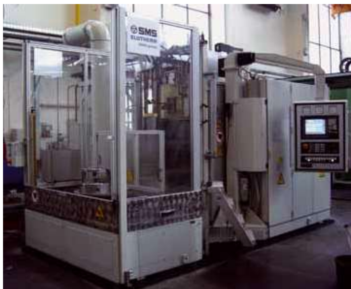
Fig. 7: Model UVH induction hardening machine, horizontally positioned ring
