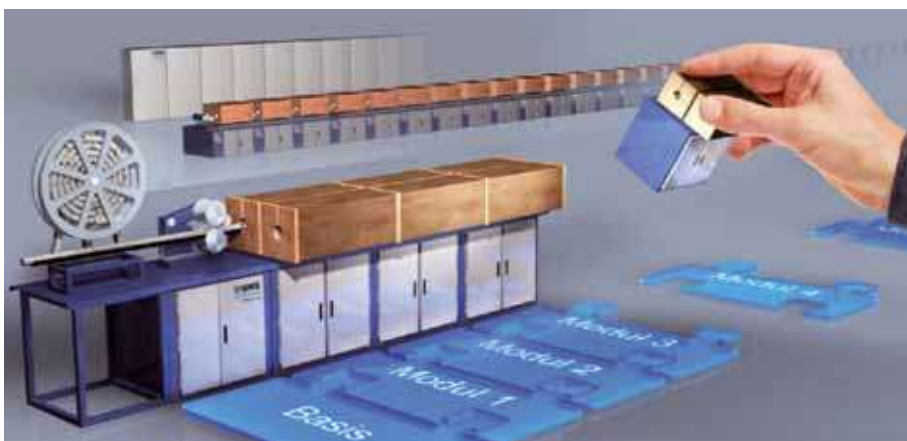
Fig. 4: Modular induction heating system
