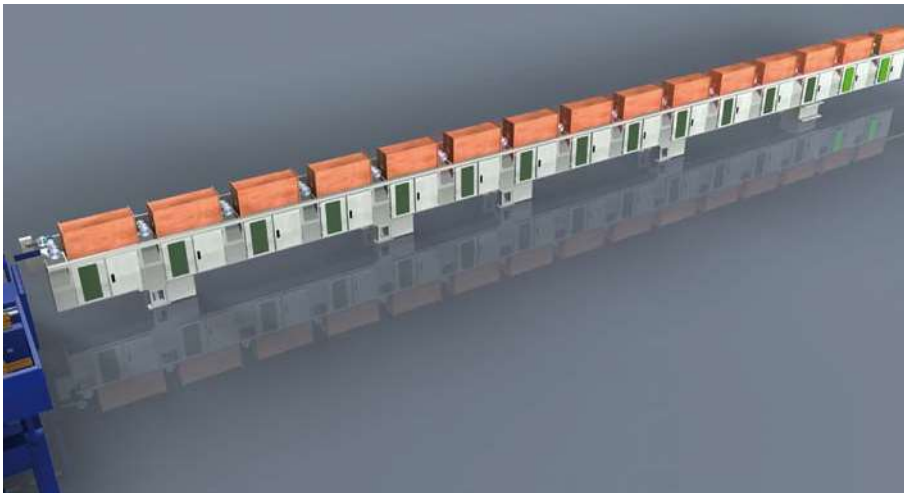
Fig. 4: Production Stop Sequence with final bar exiting the furnace (green panels indicate energized furnace zones). Each zone is automatically turned off as the bar exits
