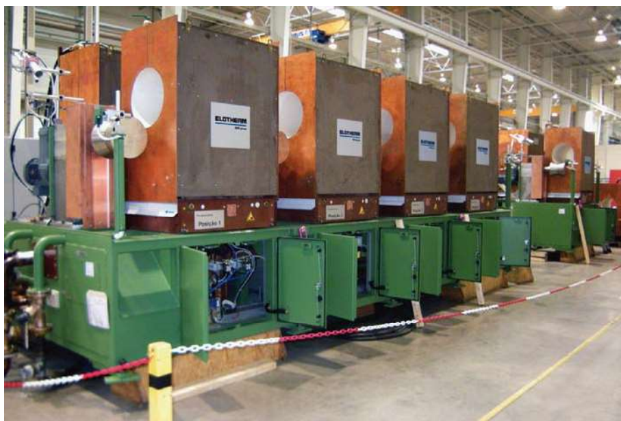
Fig. 2: High performance induction furnace for large bar heating
