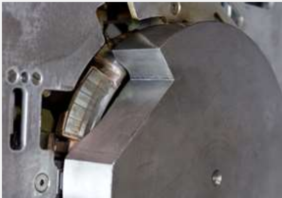
Fig. 7a: Position of the inductor in the undercut (component cut for this purpose)
