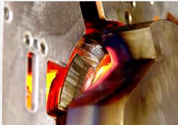
Fig. 7b: Heating pattern of the undercut inductor
