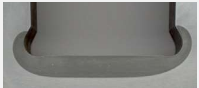
Fig. 6b: Hardening zone for two-sided undercut
