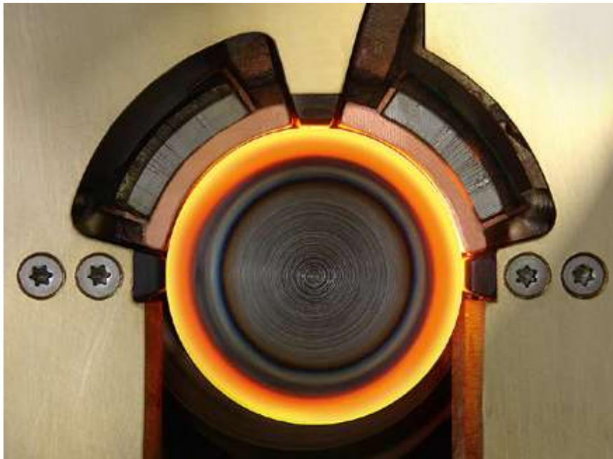
Fig. 2: Half-shell inductor for induction surface hardening of crankshafts
