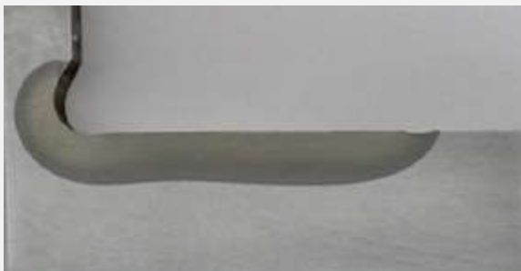
Fig. 6a: Hardening zone with single-sided undercut
