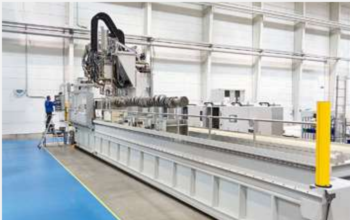
Fig. 4: EloCrank™ XL for large crankshafts (source: SMS Elotherm)
