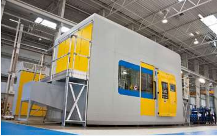
Fig. 3: EloCrank™ for automotive crankshafts (source: SMS Elotherm)
