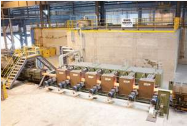
Fig. 10: SMS Elotherm EloHeat™ – induction heating plant with 6 induction coils at Tung Ho Steel in Taiwan (source: SMS Elotherm)
