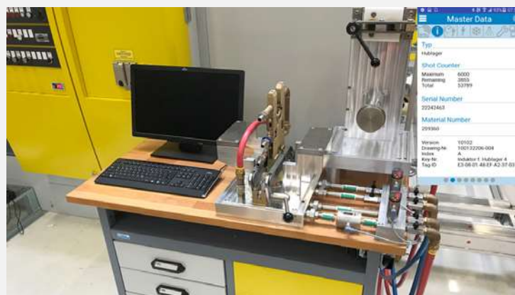
Fig. 10: Maintenance unit with flow control and PC-guided maintenance, upper right corner: screen shot of mobile phone app
